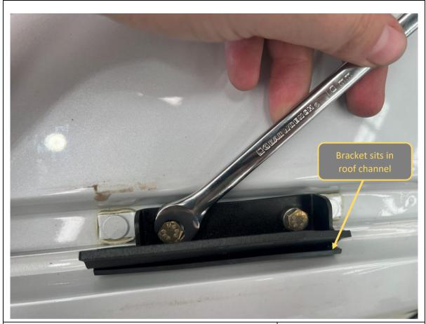
45. Ensuring the brackets are sitting correctly in the roof channel, tighten the M6 Bolts securing the FRONT mounting brackets to the roof, using a 10mm Spanner.
