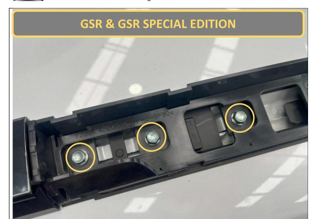
37. Using a 10mm Socket, remove the 3x bolts securing the rear mount of the roof rail to the captive nuts in the roof.
