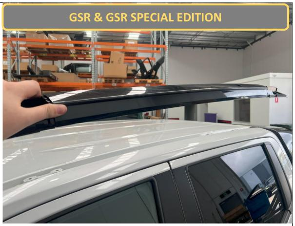
38. The roof rail should now be loose. Carefully lift the roof rail away from the car and set aside.
