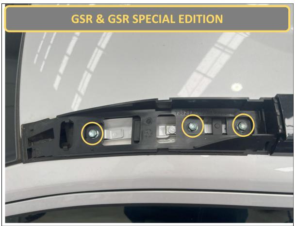
36. Using a 10mm Socket, remove the 3x bolts securing the front mount of the roof rail to the captive nuts in the roof.
