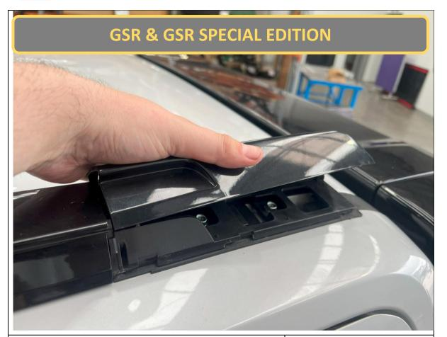
33. Using a trim tool, carefully pry up the rear roof rail cover, using similar technique to the front cover.
